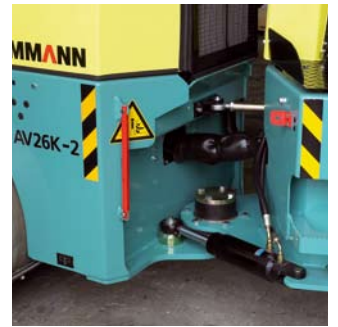
Life time lubricated central articulation joint
